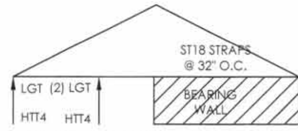
GIRDER TRUSS TYPE "G"
