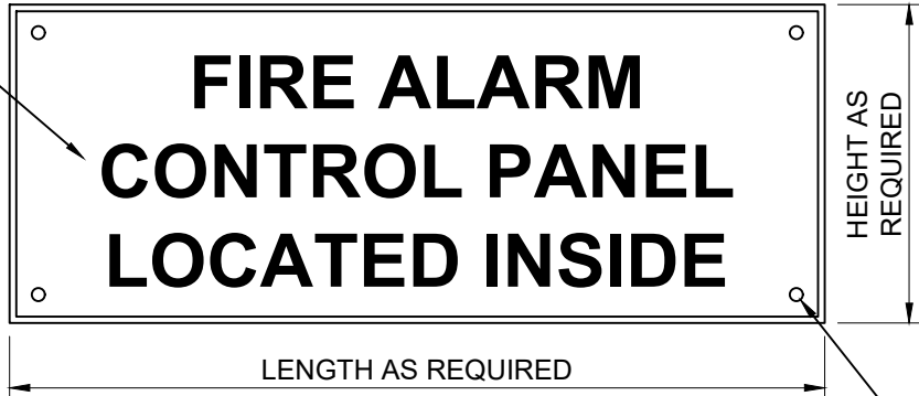
3 FACP PLACARD DETAIL NOT TO SCALE
